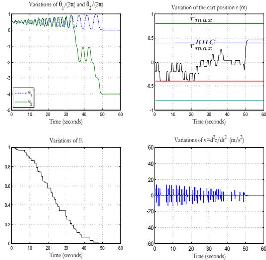
Fig. 6. Closed-loop behavior of the Twin-Pendulum systems. Initial condition  $x(0) = (0, 0, \pi, 0, \pi, 0)$ . Sampling period  $\tau_s = 0.1$  s. Maximum admissible increment on cart position  $\delta_r^{max} = 0.1$  m. This scenario is to be compared to the one depicted on figure 5 where  $\delta_r^{max} = 0.3$  m is used leading to lower response time but quite higher control level.
