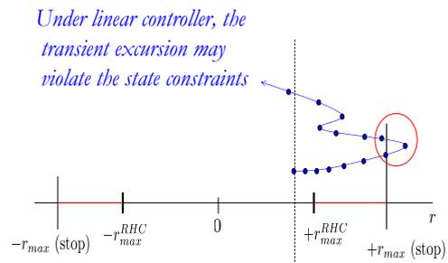
Fig. 4. Switching to the linear controller without any particular care may lead to transient state trajectories that violate the state constraints.
