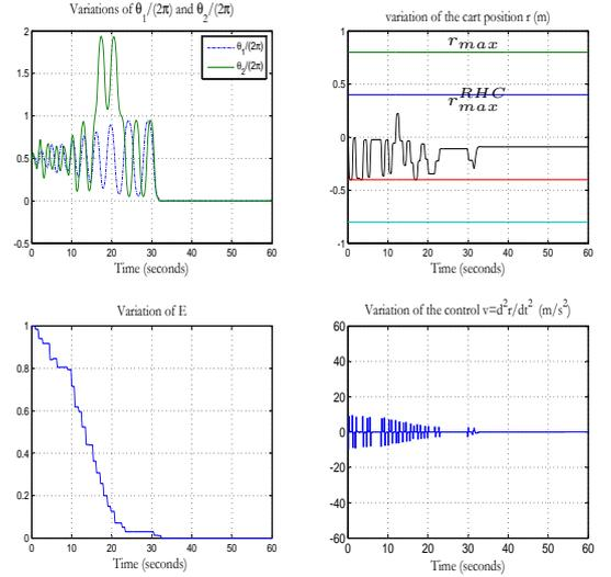
Fig. 7. Closed-loop behavior of the Twin-Pendulum systems. Initial condition  $x(0) = (0, 0, \pi, 0, \pi, 0)$ . Sampling period  $\tau_s = 0.2$  s instead of 0.1 s used in the scenarios depicted on figures 5 and 6. Maximum admissible increment on cart position  $\delta_r^{max} = 0.4$  m. Note the very low control value in comparison to figure 5 and 6 despite the fact that the maximum allowable increment is higher. This is due to the high sampling time.
