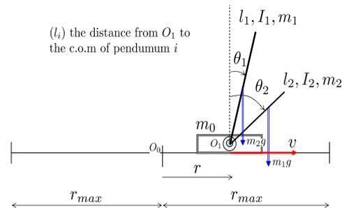
Fig. 1. View of the Twin-Pendulum system
