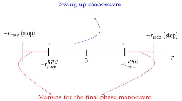
Fig. 3. Definition of the admissible domain for swing up and the margins for the final stabilization manoeuvre.
