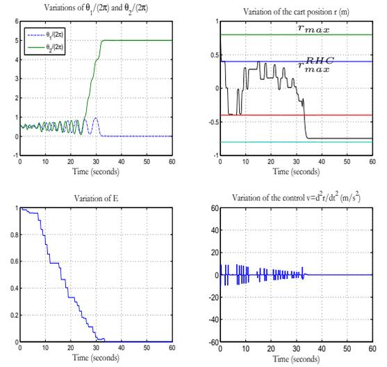
Fig. 8. Closed-loop behavior of the Twin-Pendulum systems. Initial condition  $x(0) = (0.8, 0, \pi, 0, \pi, 0)$ . Sampling period  $\tau_s = 0.2$  s. Note how the controller handles the constraint on the maximum excursion of the cart position that is initially on the boundary of the admissible region ( $r(0) = 0.8$  m)
