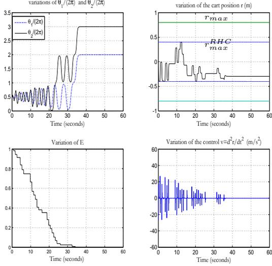
Fig. 5. Closed-loop behavior of the Twin-Pendulum systems. Initial condition  $x(0) = (0, 0, \pi, 0, \pi, 0)$ . Sampling period  $\tau_s = 0.1$  s. Maximum admissible increment on cart position  $\delta_r^{max} = 0.3$  m. This scenario is to be compared to the one depicted on figure 6 where  $\delta_r^{max} = 0.1$  m is used leading to higher response time but quite lower control level.
