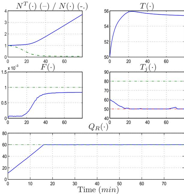
Fig. 3. Behavior of the closed loop system under the receding horizon feedback.  $Q_R^{max} = 60$ ,  $T_j^{max} = 80^\circ$ ,  $T_j^{min} = 50^\circ$ ,  $F_{max} = 0.001 \text{ mol/s}$ .  $\lambda = 1/10s^{-1}$ . Sampling period  $\tau_s = 1 \text{ min}$ .  $\varepsilon = 0.05$ . Initial conditions  $N(0) = N^T(0) = 1$ ,  $T = 50^\circ$ ,  $V(0) = 2$
