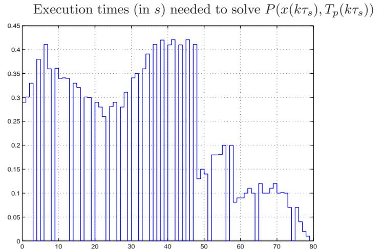
Fig. 7. The computation times needed to solve the four dimensional optimization problem at each sampling instant of the scenario depicted in Fig. 6. The upper bound of the execution times (say 0.5 s) is to be compared to the sampling period  $\tau_s = 60$  s
