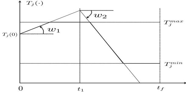
Fig. 1. Parametrization of the control input  $T_j(\cdot)$  over a time interval  $[0, t_f]$ . This parametrization is used in the definition of the receding horizon control formulation.  $T_j(\cdot)$  is defined by three parameters: the two slopes  $w_1$  and  $w_2$  that have to belong to the admissible range  $[-\dot{T}_j^{max}, \dot{T}_j^{max}]$  and the switching time  $t_1 \in [0, t_f]$ .
