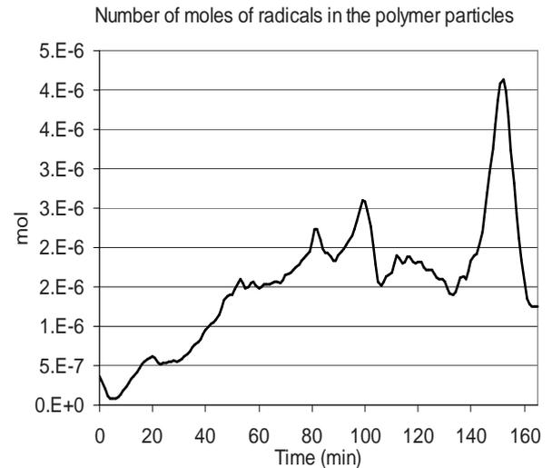
Fig. 12. Experimental validation of the controller. Number of moles of radicals in the polymer particles ( $\mu$ )
