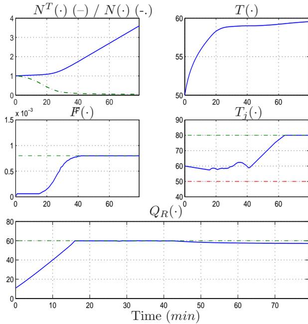
Fig. 4. Behavior of the closed loop system under the same conditions as Fig. 3 with a lower maximal allowable flow rate  $F_{max} = 0.0008$ . Note how the controller saturates the two control inputs in order to meet the achieve the control objective (remain close to the maximal allowable heat production
