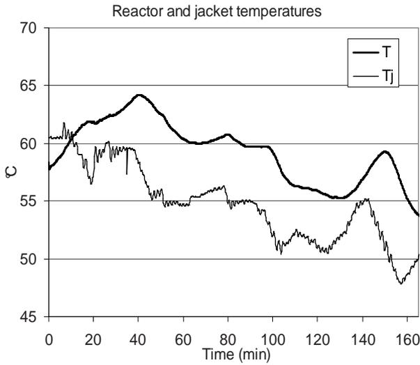
Fig. 9. Experimental validation of the controller. Reactor and jacket temperatures
