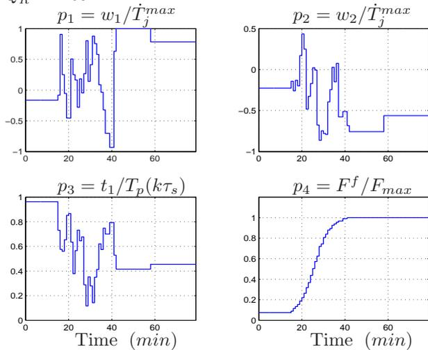
Fig. 5. Evolution of the optimal parameter vector  $\hat{p}(k\tau_s) \in \mathcal{P} \in [-1, 1]^2 \times [0, 1]^2$  during the batch depicted on Fig. 4.
