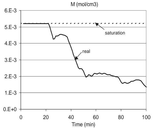
Fig. 11. Experimental validation of the controller. Concentration of monomer in the polymer particles
