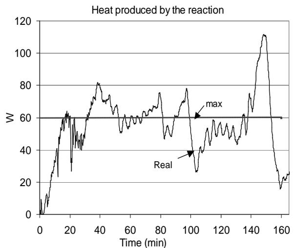
Fig. 8. Experimental validation of the controller. The heat produced by the reaction with a maximal constraint at 60 W
