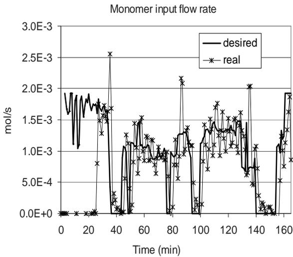
Fig. 10. Experimental validation of the controller. Controlled monomer flow rate and the reaction rate
