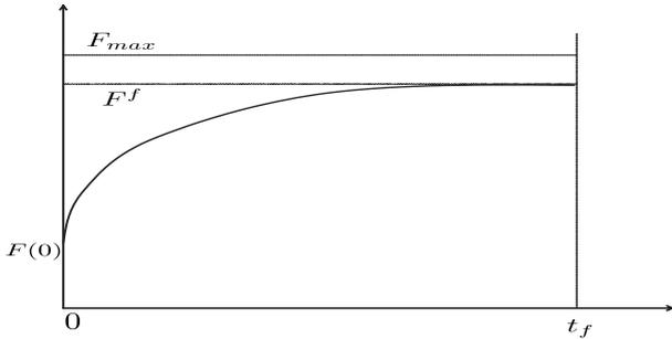
Fig. 2. Parametrization of the control input  $F(\cdot)$  over a time interval  $[0, t_f]$ . This parametrization is used in the definition of the receding horizon control formulation.  $F(\cdot)$  is defined by one parameter, namely its asymptotic value  $F^f$ .
