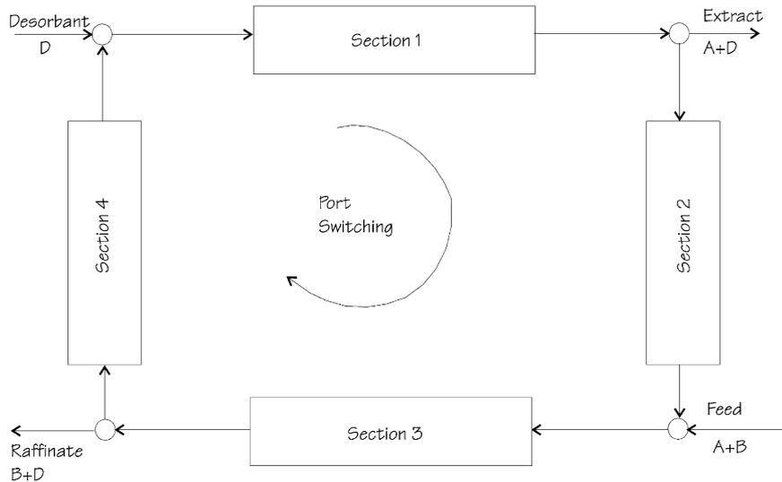
Fig. 1. Schematic view of a simulated moving bed.
