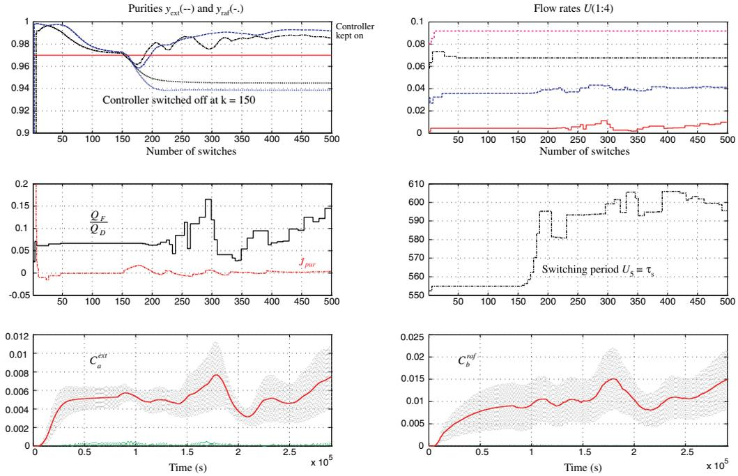
Fig. 6. Response of the controlled/uncontrolled SMB to a unmeasured  $-10\%$  step change of the void fraction  $\varepsilon$ .
