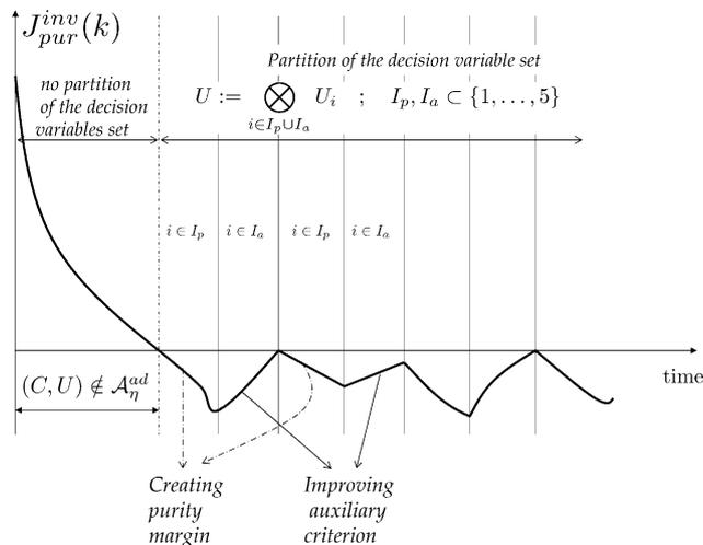
Fig. 2. Schematic view of the control algorithm.
