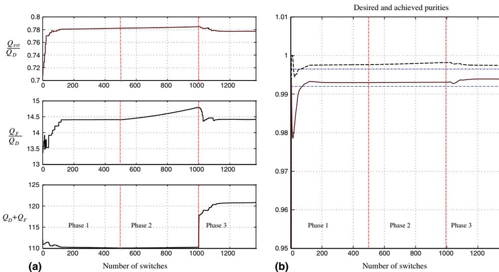
Fig. 7. Scenario 1, High separation SMB. (a) The purities and their set point  $y_d = (0.992, 0.997)$ . (b) The different cost functions fired at different instants during the scenario. Note how the controller takes into account the sudden changes in the fired auxiliary cost and increases appropriately the corresponding value while keeping the purities above the required set-points.
