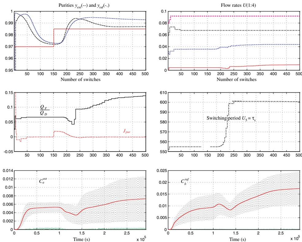
Fig. 3. Response of the controlled SMB to a step change of the desired purities  $y_d$ :  $y_d$  changes at  $k = 150$  from  $(0.97, 0.97)$  to  $(0.99, 0.99)$ .
