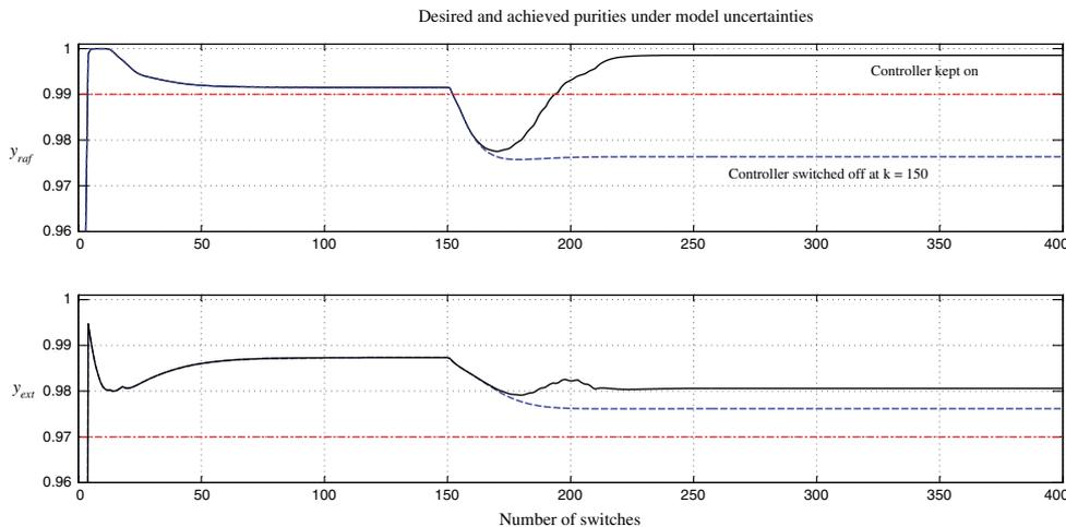
Fig. 8. Behaviour of the closed loop system (continuous line) and the system with the controller switched off after the 150th switch (dotted line) in the presence of +1.8% unmeasured step change of the Langmuir coefficients.
