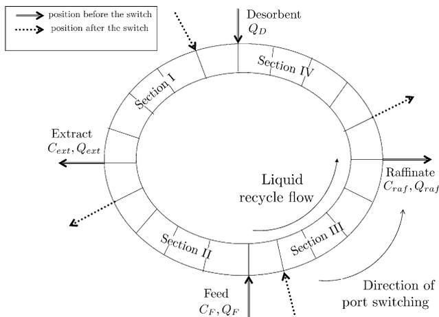
Fig. 1. Schematic view of a simulated moving bed.
