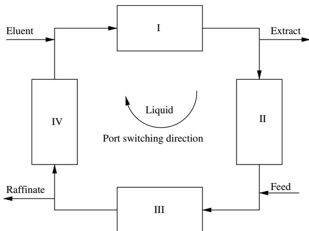
Fig. 1. Scheme of the simulated moving bed.
