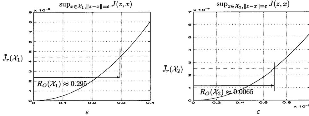
Fig. 3. Computation of the Observability radius for system (13) for  $\mathcal{X} = \mathcal{X}_1$  and  $\mathcal{X} = \mathcal{X}_2$ .
