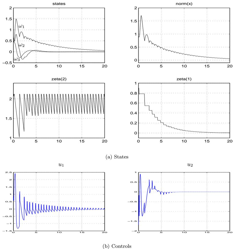
Figure 2: Stabilization of the angular velocities of the rigid body. The free-disturbance case
