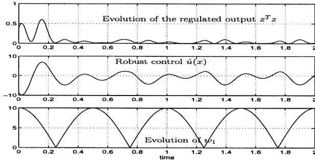
Fig. 2. Closed loop behaviour under external disturbances  $w_1$  for Example 5.2—initial state  $x_0 = (0.5, 0.15, -0.6)^T$ .
