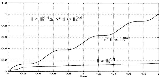
Fig. 3. Test of the  $H_\infty$  attenuation inequality for Example 5.2—initial state  $x_0 = (0.5, 0.15, -0.6)^T$ .
