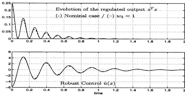
Fig. 1. Closed loop behaviour under parameter uncertainties for Example 5.2.
