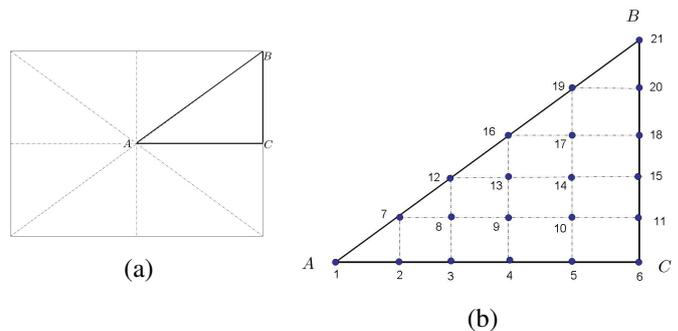
Fig. 3. (a) Because of symmetry, only the triangle  $ABC$  is considered. (b) The set of different positions where measurements are acquired for design and/or validation
