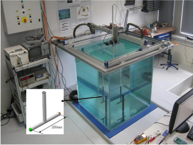
Fig. 1. Photo of the experimental facility available at SUBATECH. One can recognize the position/orientation control plate-form for the electro-sensor probe. This enables a controlled movement of the probe in the aquarium to be performed in order to collect the resulting electro-sensing measurements.
