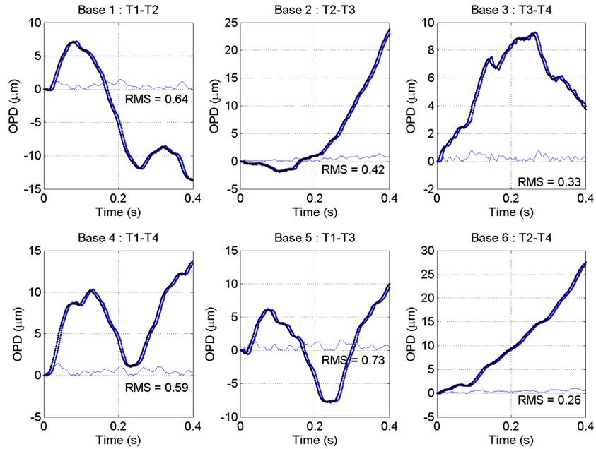
Figure 6. Simulation results with  $N = 4$  and  $B = 6$ . Control loop with piston observer order 1, but no take into account of delay. Black : setpoint (piston); Blue : OPD between DLs; Blue thin : residual OPD
