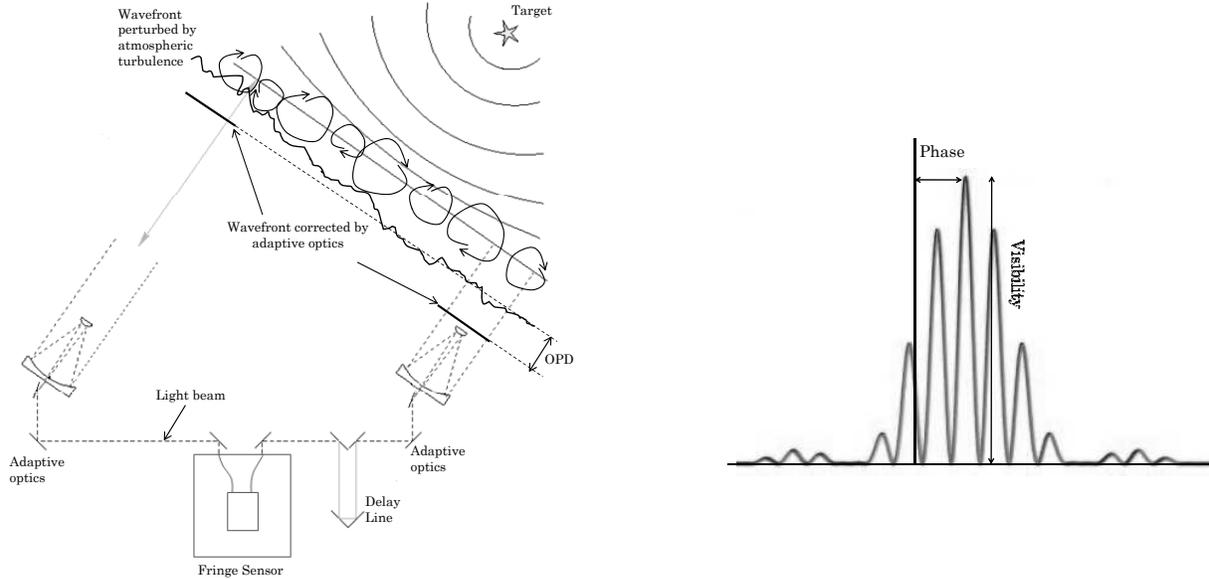
Figure 1. Left : Problematic of the piston OPD. Right : the two observables on interference fringes
