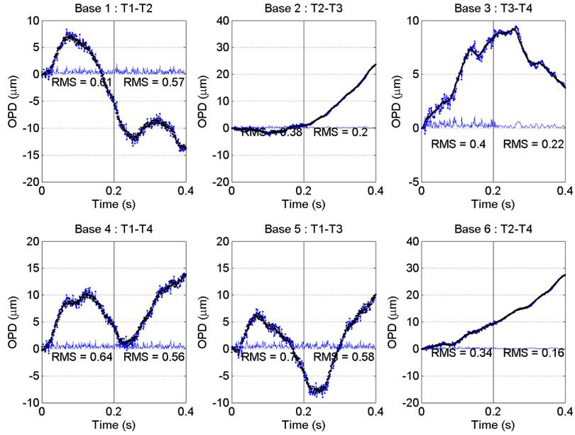
Figure 9. Simulation of a loss of flux from the telescope 1, with  $N = 4$  and  $B = 6$ . Measures from the three bases affected by this telescope are more noised. During the first half the weighting is off, and it's on during the second one. Control loop with piston observer order 3. Black : setpoint (piston); Blue : OPD between DLs; Blue thin : residual OPD
