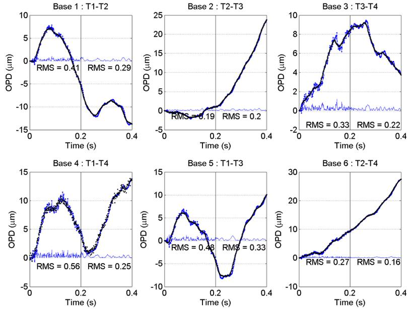
Figure 10. Simulation of a drop out of visibility on the base 4, with  $N = 4$  and  $B = 6$ . Measures from this bases is more noised. During the first half the weighting is off, and it's on during the second one. Control loop with piston observer order 3. Black : setpoint (piston); Blue : OPD between DLs; Blue thin : residual OPD
