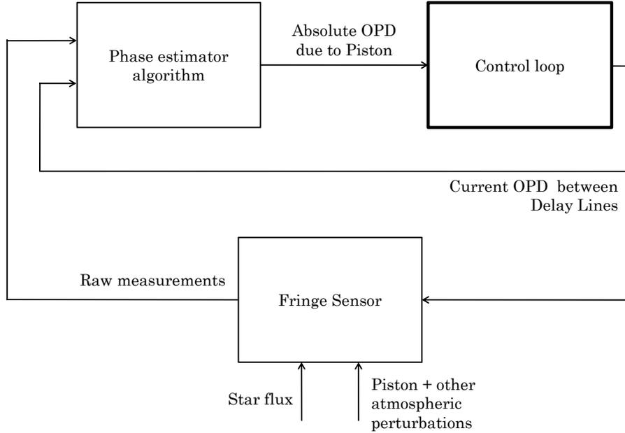
Figure 2. Scheme of a fringe tracker loop
