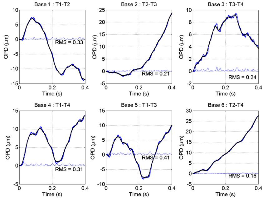
Figure 8. Simulation results with  $N = 4$  and  $B = 6$ . Control loop with piston observer order 1. Black : setpoint (piston); Blue : OPD between DLs; Blue thin : residual OPD
