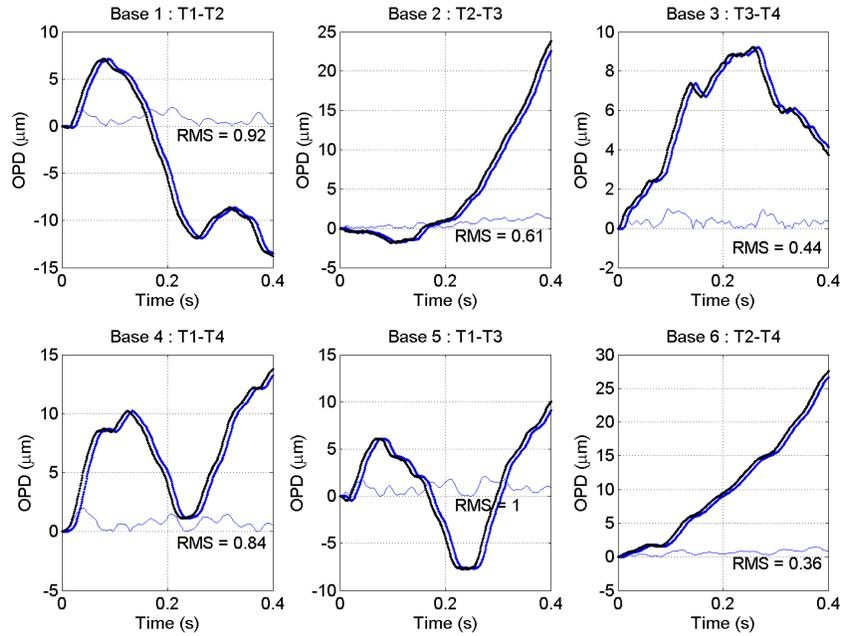
Figure 7. Simulation results with  $N = 4$  and  $B = 6$ . Control loop without piston observer. Black : setpoint (piston); Blue : OPD between DLs; Blue thin : residual OPD
