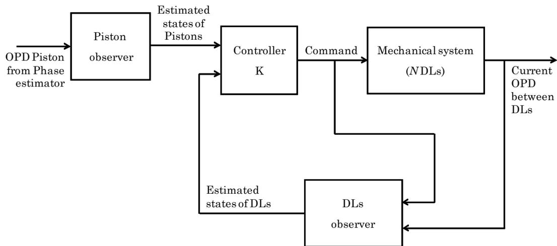
Figure 4. Scheme of control loop
