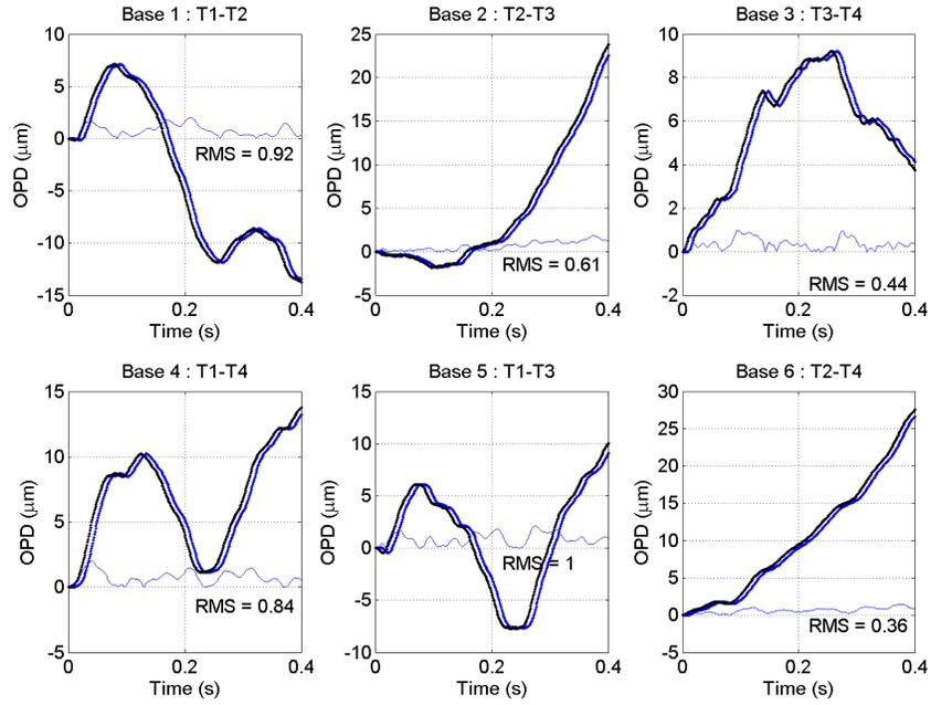
Figure 5. Simulation results with  $N = 4$  and  $B = 6$ . Control loop with piston observer order 0, but no take into account of delay. Black : setpoint (piston); Blue : OPD between DLs; Blue thin : residual OPD
