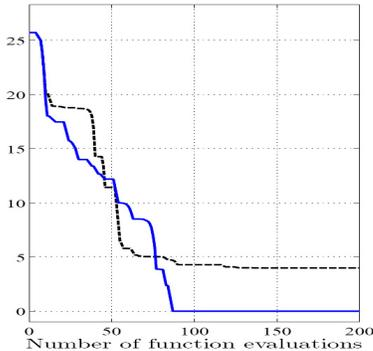
Fig. 6. Evolution of the cost functions  $\bar{\Delta}_0^{0.3}(q)$  [black dotted] and  $\bar{\Delta}_7^{0.3}(q)$  [blue solid] during the optimization of the excitation vector  $q$ . Note that in the absence of redundancy use, no solution can be found that achieves the contraction factor  $\gamma = 0.3$
