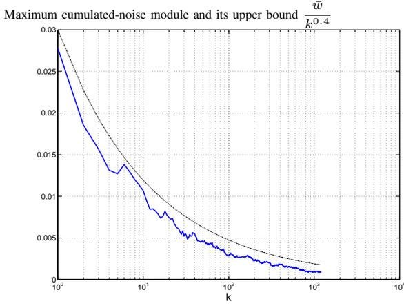
Fig. 3. Identification of the noise characterization parameters  $\bar{w}$  and  $\phi_w(\cdot)$ . 1000 runs of the MATLAB function RANDN are used. Each run contains  $20 \times k_{max} = 1200$  samples. For each  $k \in \{1, \dots, 20 \times k_{max}\}$ , the maximum over these runs of the absolute value of the cumulated noise is plotted (blue continuous line) versus its suggested upper bound  $\phi_w(k)\bar{w}$  (black dotted line) with  $\bar{w} = 0.0031$  and  $\phi_w(k) = 1/k^{0.4}$ .
