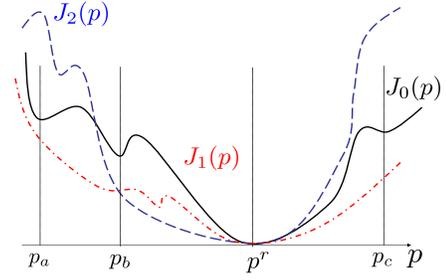
Fig. 1. Typical scheme for a 2-safely redundant optimization problem defined by the cost function  $J_0$ .  $J_0$  (in black-solid line) admits one global minimum  $p^r$  and 3 local minima  $p_a$ ,  $p_b$  and  $p_c$ . However, the singularities  $p_a$  and  $p_c$  can be crossed following the  $(p_a, J_1)$  and the  $(p_b, J_1)$ -solver paths respectively while the singularity  $p_b$  can be crossed following the  $(p_b, J_2)$ -solver path.
