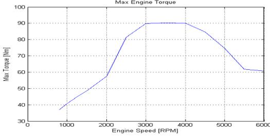
Fig. 2. Maximum engine torque  $\mathcal{T}(\omega_e)$  vs engine speed
