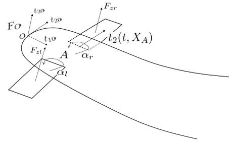
Fig. 2. Pectoral fins positions and the induced forces
