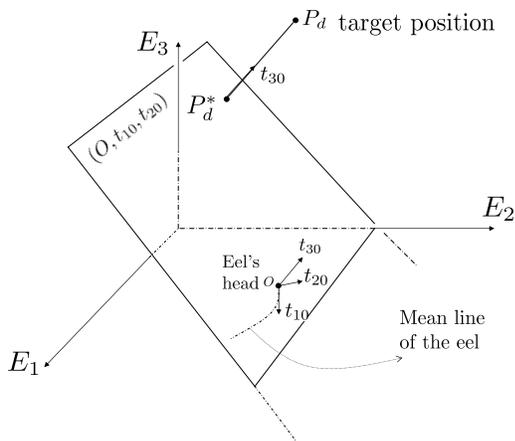
Fig. 3. Schematic 3D view of the control problem. The Eel that lies at instant  $t$  in the plane  $(0, t_{10}(t), t_{20}(t))$  has to join the target position  $P_d$  while trying to keep the vector  $t_{20}$  horizontal, namely  $t_{20} \cdot E_3 \approx 0$ . This has to be done using the infinite dimensional control input  $(K(\cdot, \cdot), \alpha_r, \alpha_l)$ .
