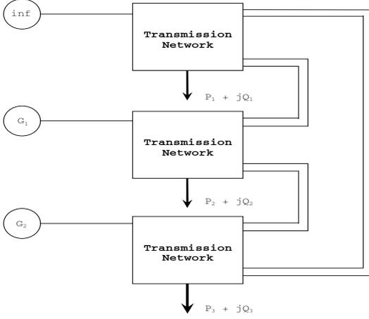
Fig. 1. The ABB medium scale benchmark
