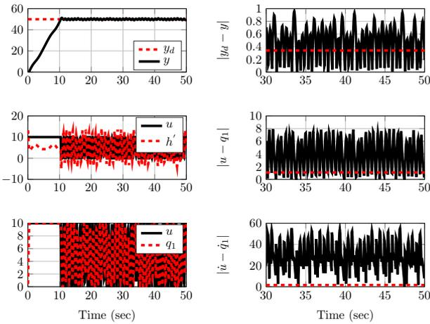
Fig. 4. Closed loop simulation results for  $\lambda = 10$  and  $\lambda_f = 1.1$ , where red dotted lines on plots on the right side represent upper bounds computed by (33),(10) and (11) respectively.
