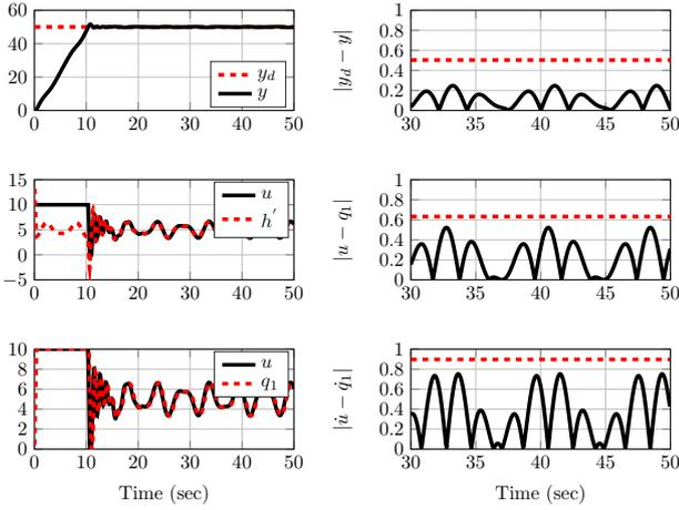
Fig. 3. Closed loop simulation results for  $\lambda = 5.6$  and  $\lambda_f = 1.1$  (optimal solution), where red dotted lines on plots on the right side represent upper bounds computed by (33),(10) and (11) respectively.
