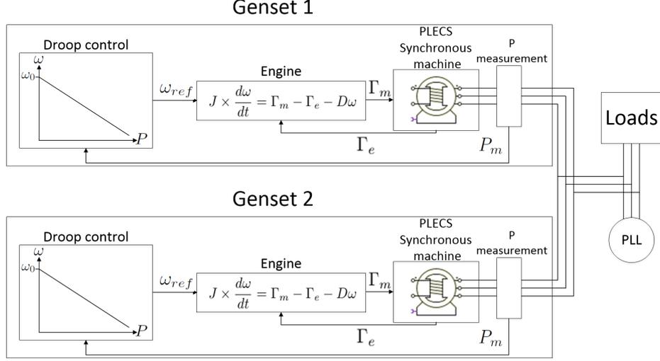
Figure 3. Schematic view of the simulation used to identify the two-gensets grid frequency dynamics.
