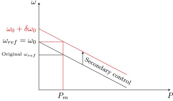
Figure 7. Droop with secondary control
