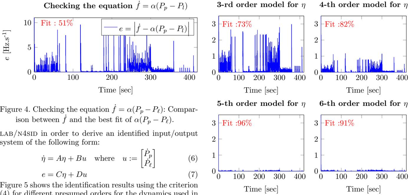
Figure 4. Checking the equation  $\dot{f} = \alpha(P_p - P_l)$ : Comparison between  $\dot{f}$  and the best fit of  $\alpha(P_p - P_l)$ .
