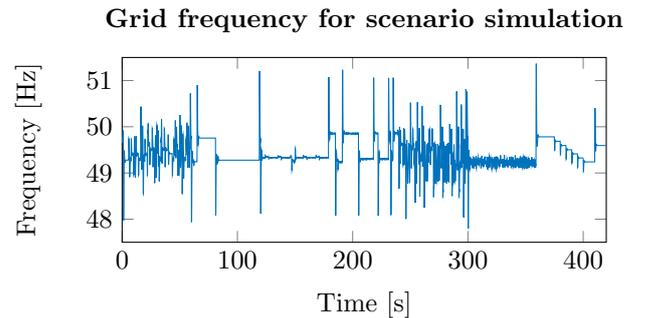
Figure 2. The frequency evolution during the identification scenario in response to the active power load profile of Figure 1.
