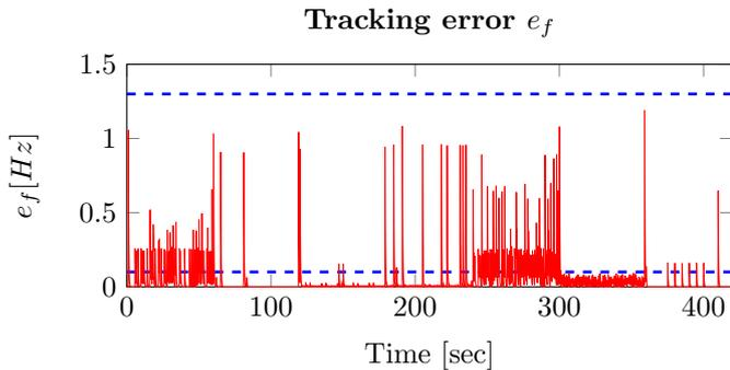
Figure 11. Tracking error of closed-loop of (9) and (11) with  $\lambda = 1120$  and  $\lambda_f = 34$ . Dotted lines represents the bounds 1.3 and 0.1 corresponding to continuously varying  $P_\ell$  and  $\dot{P}_\ell = 0$
