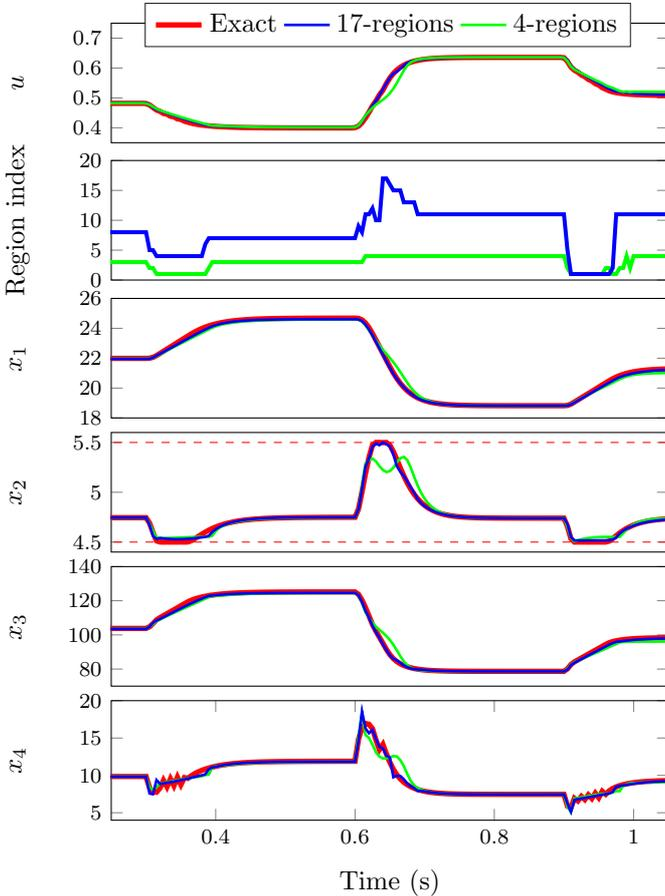
Fig. 4. Performance comparison between controllers
