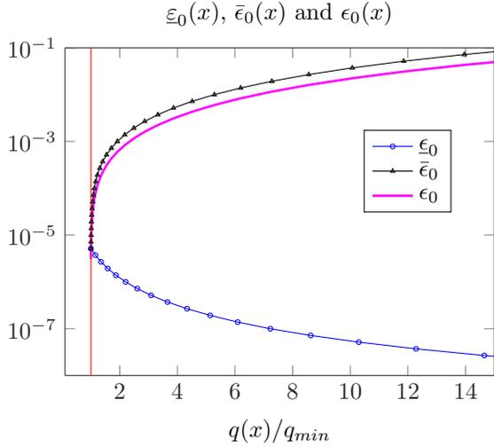
Fig. 4. Typical evolution of the state-dependent targeted precision  $\epsilon(x)$  leading to the state-dependent control updating period  $\tau(x) := [\tilde{m}(\epsilon_0(x), \tau_c)] \tau_s$ . Example of a chain of integrator system (Alamir (2015)).
