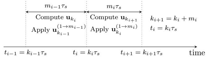
Fig. 1. The real-time implementation scheme: Definition of the control updating instants  $t_i = k_i\tau_s$ .
