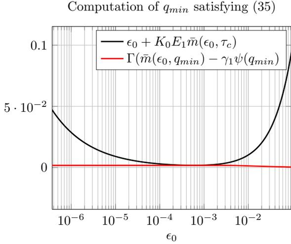
Fig. 5. Instantiation of Figure 3.(c) in the case of the triple integrator example. Satisfaction of the fundamental inequality (35) for  $q_{min} = 0.051$ . The computation time  $\tau_c = 10\mu s$  is considered for a single iteration of the fast gradient algorithm.
