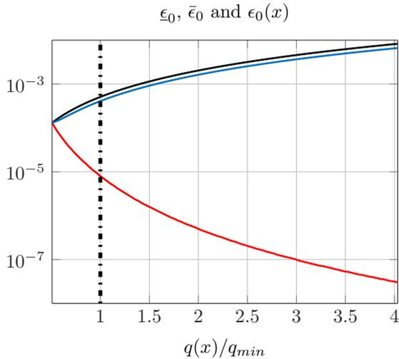
Fig. 6. Resulting state dependent targeted precision  $\epsilon_0(x)$  for the triple integrator example with  $\tau_c = 10\mu s$ .
