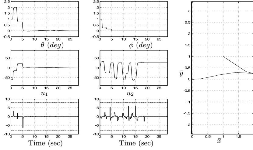
**Fig. 4.** Closed loop behavior. Initial condition  $\bar{x}(0) = \bar{y}(0) = 1$ ,  $\theta(0) = -\pi/4$  and  $\xi(0) = 0$ . Saturation levels  $u_1^{max} = u_2^{max} = 8$ . This figure is to be compared with figure 5 in order to appreciate the saturation constraints handling.
