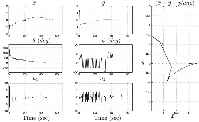
**Fig. 9.** Closed loop behavior. Initial condition  $\bar{x}(0) = -1$ ,  $\bar{y}(0) = 1$ ,  $\theta(0) = 3\pi/4$  and  $\xi(0) = 1$ . Saturation levels  $u_1^{max} = u_2^{max} = 8$ . The uncertainties given by (37)-(38) are used to test the robustness of the proposed feedback algorithm.
