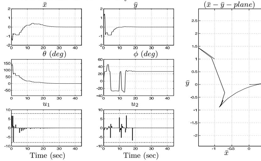
**Fig. 8.** Closed loop behavior. Initial condition  $\bar{x}(0) = -1$ ,  $\bar{y}(0) = 1$ ,  $\theta(0) = 3\pi/4$  and  $\xi(0) = 1$ . Saturation levels  $u_1^{max} = u_2^{max} = 8$ . This simulation is done under nominal model without uncertainties. The result is to be compared to that of figure 9 where model uncertainties are introduced.
