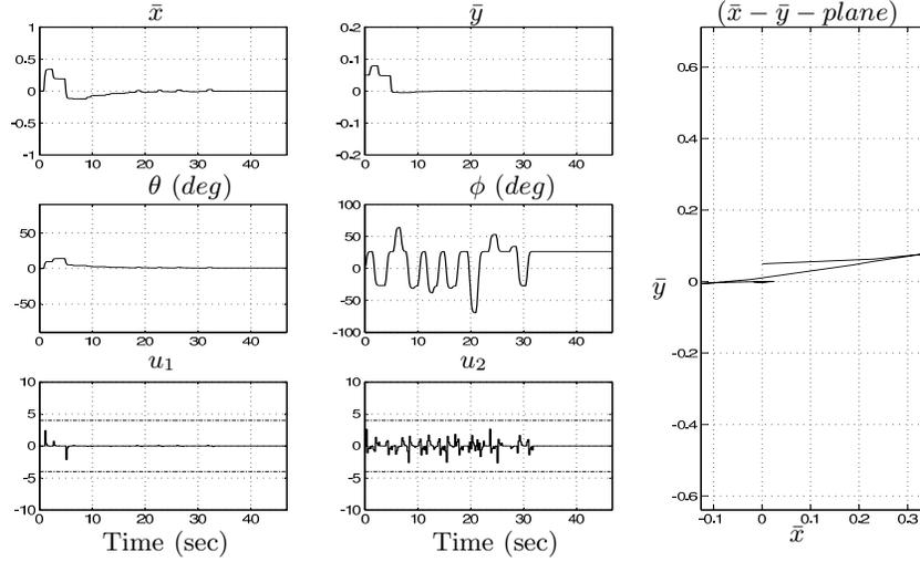
**Fig. 6.** Closed loop behavior. Initial condition  $\bar{x}(0) = 0$ ,  $\bar{y}(0) = 0.05$ ,  $\theta(0) = 0$  and  $\xi(0) = 0$ . Saturation levels  $u_1^{max} = u_2^{max} = 4$ . Note how the parametrization of the trajectories avoids the need for a whole rotation even in this rather singular situation.
