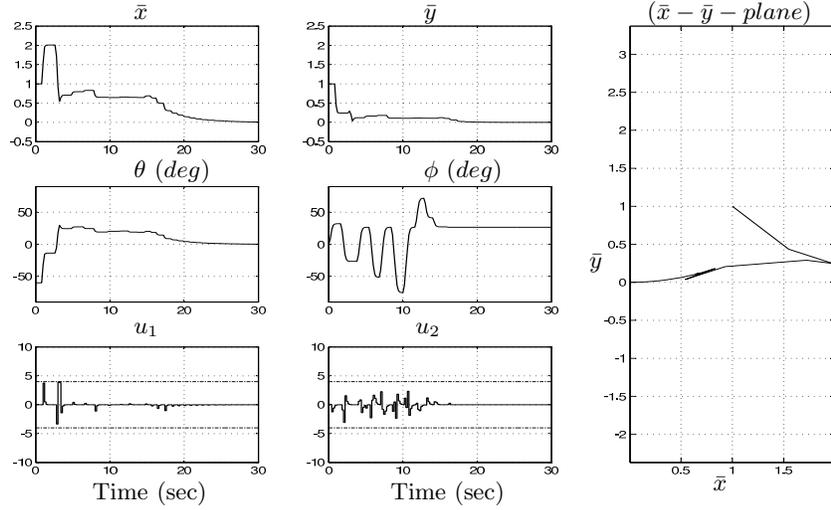
**Fig. 5.** Closed loop behavior. Initial condition  $\bar{x}(0) = \bar{y}(0) = 1$ ,  $\theta(0) = -\pi/4$  and  $\xi(0) = 0$ . Saturation levels  $u_1^{max} = u_2^{max} = 4$ . This figure is to be compared with figure 4 in order to appreciate the saturation constraints handling.
