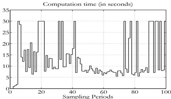
**Fig. 5.** Computation times needed to achieve the state estimation depicted on figure 3. Note that an explicit upper bound has been imposed in the internal loop of the optimizer in order to deliver the best estimation that can be obtained within the available computation time defined by the sampling period (30 seconds). This scenario uses a tolerance  $\varepsilon = 10^{-8}$  for the optimization subroutine.
