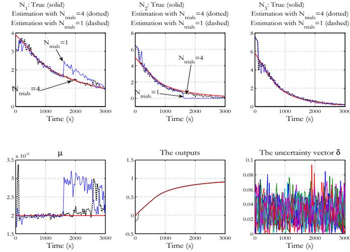
**Fig. 4.** Comparison between the observer behavior when  $N_{trials} = 1$  and  $N_{trials} = 4$  under the scenario depicted on figure 3. Note how the singularity cross mechanism enables to avoid drops in the estimation quality when the observer encounters a singular situation. This scenario uses a tolerance  $\varepsilon = 10^{-8}$  for the optimization subroutine.
