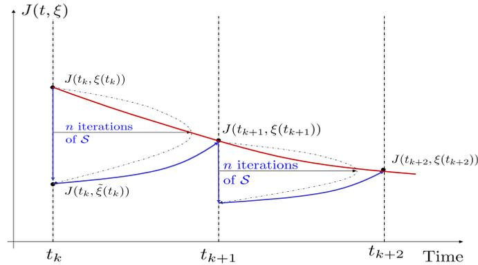
**Fig. 15.** Schematic view of the distributed-in-time optimization based observer. Note that the convergence of the overall estimation scheme is the result of a competition between a decreasing effect due to the optimizer and the increasing effect due to the natural divergence of open-loop state estimation.
