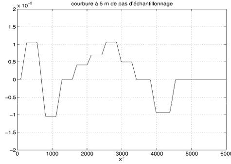
**Fig. 10.** Evolution of the curvature map  $\rho(\cdot)$  on a portion of the Paris-Toulouse line. This map is used in the validating scenarios.
