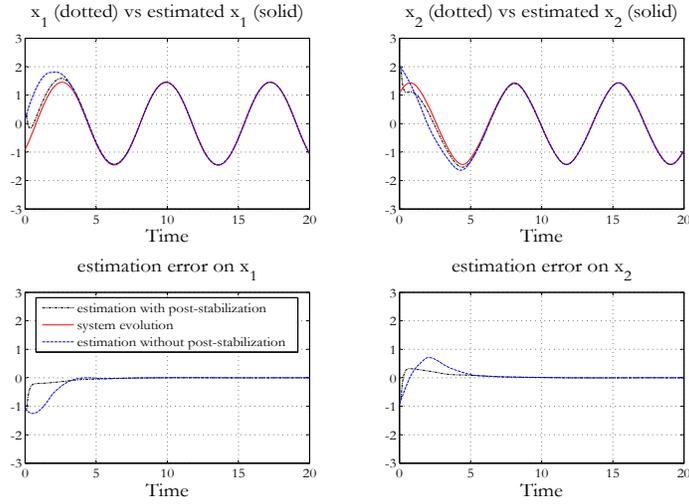
**Fig. 13.** Comparison between moving-horizon observer with (black dot-dashed line) and without (dotted) post-stabilization step. Here, the updating period is  $\tau_s = 0.1$  s. This is sufficiently small to make the moving-horizon observer stabilizing even without the post stabilization step. Even in this case, note how the post stabilization step improves the quality of the estimation.
