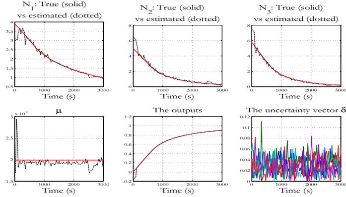
**Fig. 2.** Observer behavior under model uncertainty given by (39)-(43) with  $d_{max} = 10\%$  and no measurement noise ( $\nu_{max} = 0$ ). The observation horizon is  $N = 10$  and the number of trials for the singularity crossing scheme is  $N_{trials} = 4$ . Initial state of the observer is  $\hat{x}(0) = \text{diag}(0.8, 1.3, 1.3) \cdot x(0)$  and  $\mu_{obs}(0) = 0.8\mu_{model}$ .
