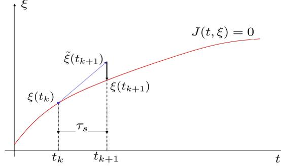
**Fig. 8.** The post-stabilization technique. To obtain the next observer state  $\xi(t_{k+1})$ , the observer equation is first integrated using constant gradient term  $J_\xi(t_k, \xi(t_k))$ , then the result  $\tilde{\xi}(t_{k+1})$  is projected on the sub-manifold  $J(t_{k+1}, \xi) = 0$ .
