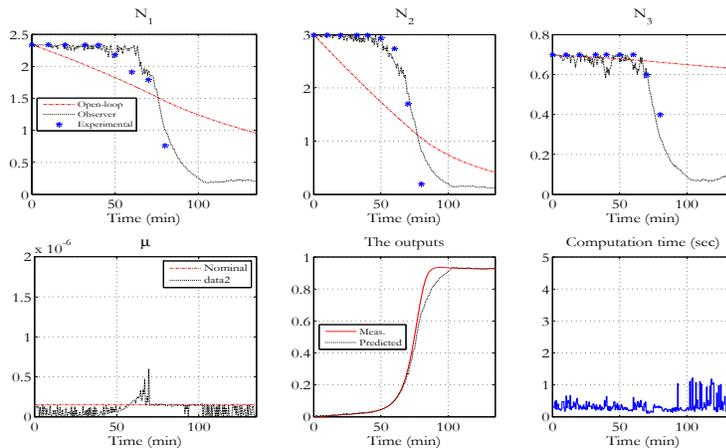
**Fig. 7.** Results under the same experimental validation scenario as figure 6 with  $N_{trials} = 1$  and tolerance threshold  $\varepsilon = 10^{-3}$ . Note the slight drop in the estimation quality (particularly on  $N_2$ ) compared to figure 6 where the singularity cross technique is used.
