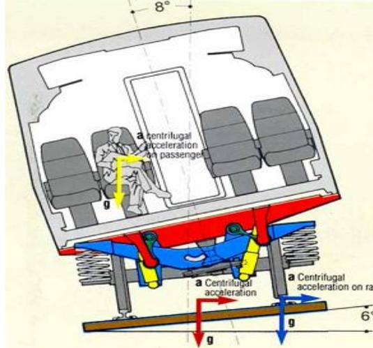
**Fig. 9.** Schematic view of a tilting train. The additional control-induced inclination of the compartment allows for a higher speed on existing rails while keeping the same comfort level (by maintaining the resulting felt acceleration normal to the compartment floor).
