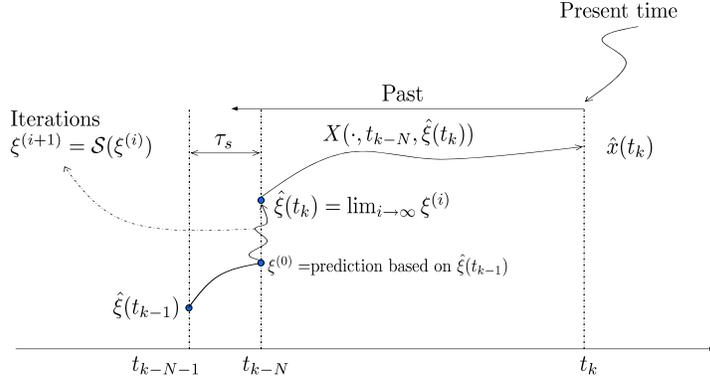
**Fig. 1.** Ideal computation scheme to solve the optimization problem (20). The iterative process  $\mathcal{S}$  is initialized at  $\xi^{(0)}$  that is obtained using the past estimated value  $\hat{\xi}(t_{k-1})$ . Then, the iterations ideally lead asymptotically to the solution  $\hat{\xi}(t_k)$ . Integrating the system equations enables the computation of the current estimation  $\hat{x}(t_k)$ .
