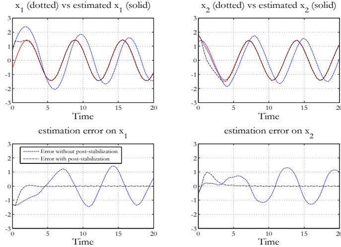
**Fig. 14.** Comparison between moving-horizon observer with (black dot-dashed line) and without (dotted) post-stabilization step. Here, the updating period is  $\tau_s = 0.4$  s. Note how the post stabilization step enables the updating period to be increased while maintaining good precision.
